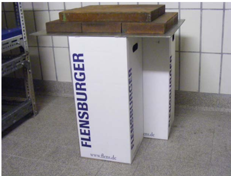
Image 8: Test container with an axial loading of 400 N per container
